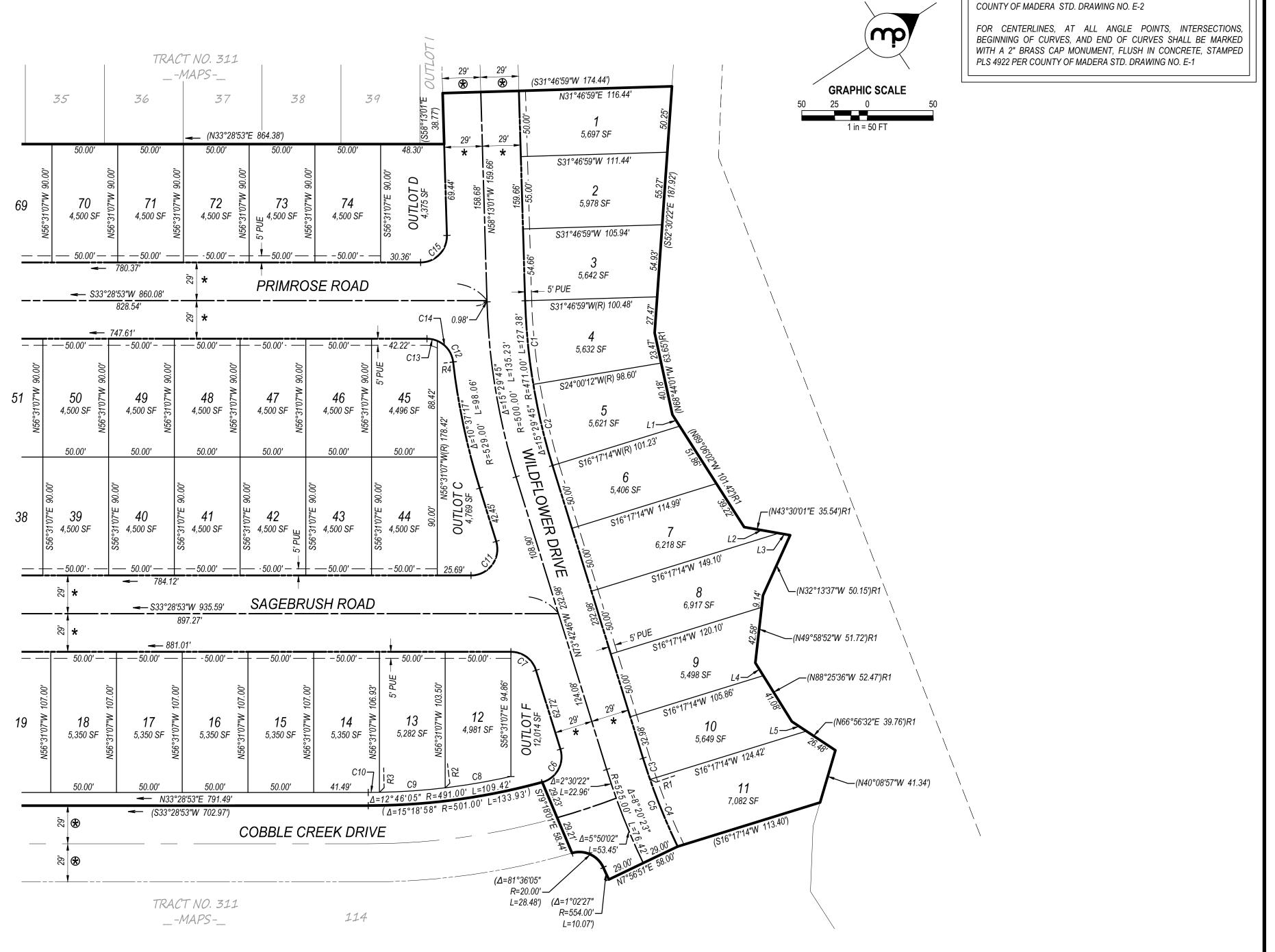
FOR LOT BOUNDARIES, AT ALL LOT CORNERS, ANGLE POINTS, INTERSECTIONS, BEGINNING OF CURVES, AND END OF CURVES SHALL BE MARKED WITH A 3/4" IRON PIPE, DOWN 6", TAGGED PLS 4922 PER COUNTY OF MADERA STD. DRAWING NO. F-2
