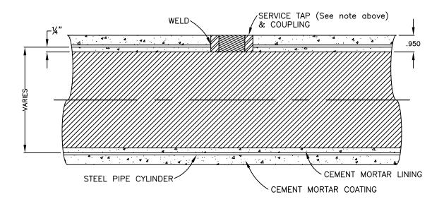
ALL WATER SERVICE TAPS FOR CEMENT — COATED STEEL PIPE SHALL BE SHOP FABRICATED.
