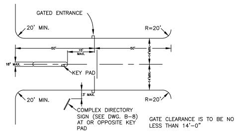
KEY SWITCH TO BE MOUNTED ON EXTERIOR, EITHER ON STEEL GOOSENECK OR ON WALL OR GATE POST WITHIN 3' OF ROADWAY AND NOT OVER 15' FROM GATE.
