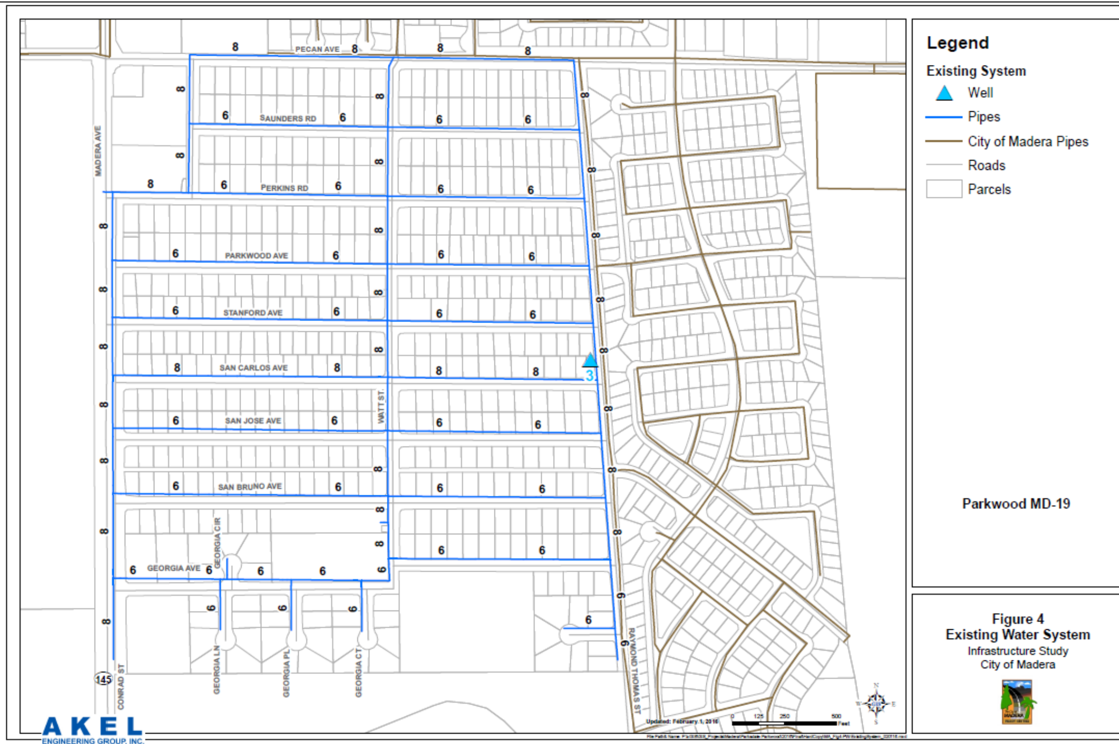
Figure 6-2 MD-19 Water System (Akел Engineering Group, Inc., 2016)
